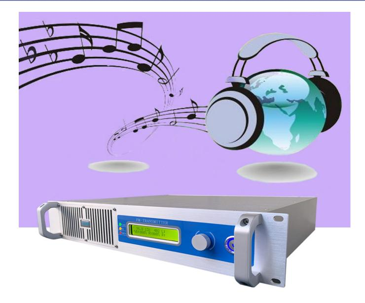
The transmitter implements digital FM modulator module as its core, combining with RF power amplifier. In the transmitter, DSP&DDS are used to execute all-digital processing, such as digital filtering, pre-emphasis, the generation of pilot frequency, stereo coding and FM modulating. A AGC circuit is used to keep the set power stable.
